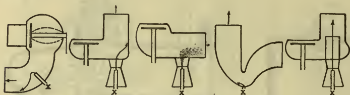
FIG. 171.—A few examples of carburetter design, showing courses followed by the fuel after leaving the nozzle, for different arrangements of parts and passages. The heavy arrowed line leading from the nozzle X indicates the course taken by the mixture as influenced by the design. These diagrams are self explanatory, and show that liquid globules are precipitated against some portions of the mixing chamber wall almost immediately after leaving the nozzle. This tends to disturb the homogeneity of the mixture, and requires that provisions be made for correcting this effect in the remaining portions of the passage.
